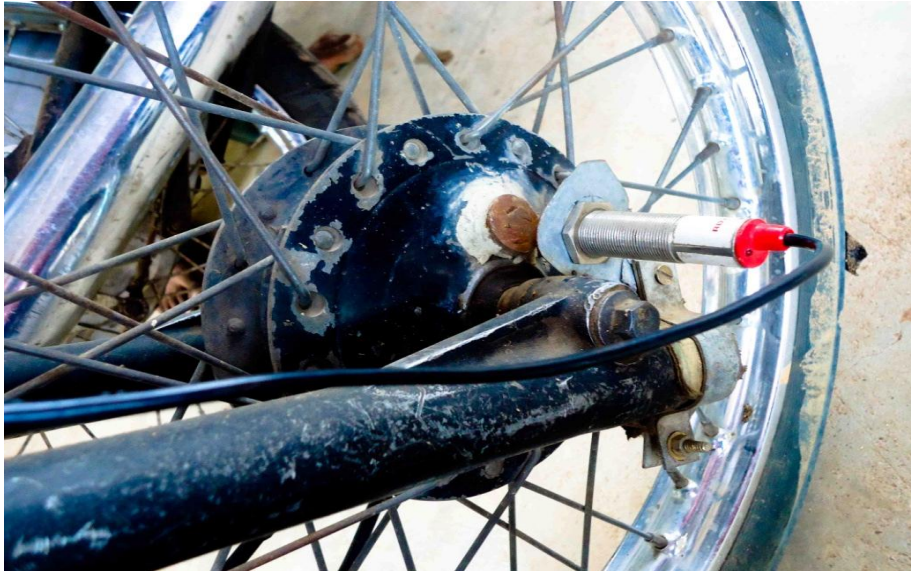
Fig. 14: Inductive speed sensor mounting
